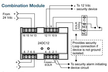
Optional - 24Vdc power used with ground isolating option.
